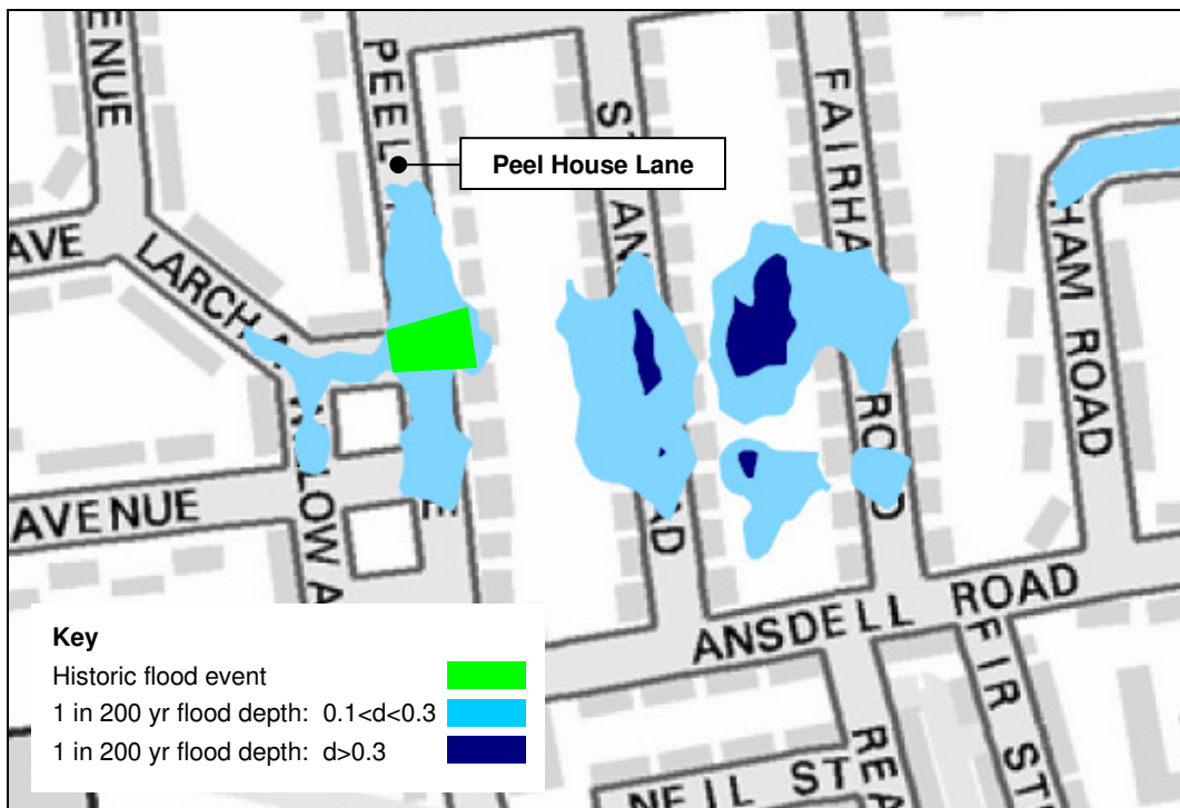
Figure 3.1: Comparison of historic flooding event with modelled surface water flooding on Peel House Lane (extract from Drawing 282945/NWD/MCH/101)
