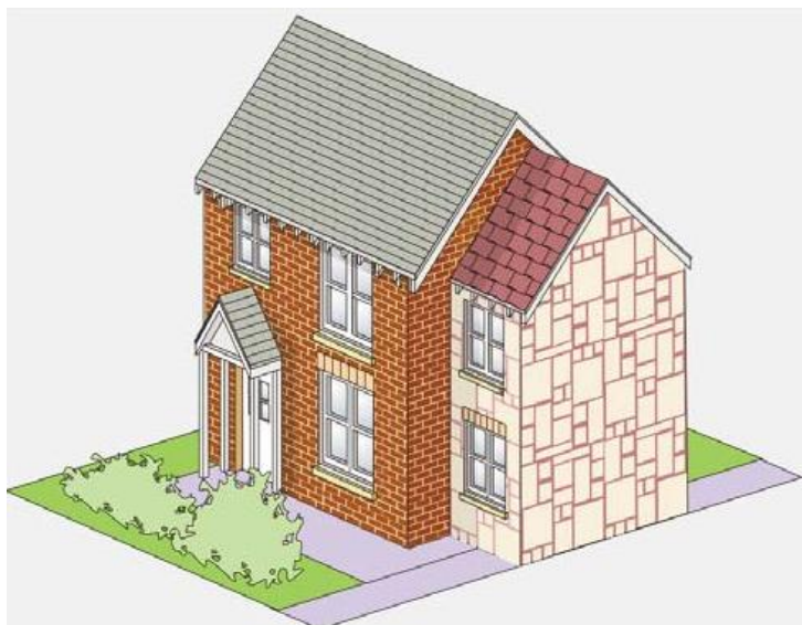
Diagram 3: Poor choice of external materials for the extension.
