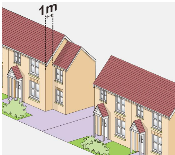
Diagram 13: Good side extension. Set back 1m and with lower ridge height.
