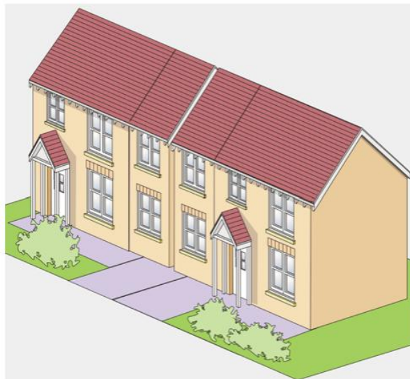
Diagram 14: Inappropriate side extensions which have led to a 'terracing effect'.
