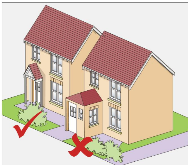
Diagram 11: Inappropriate porch extension
