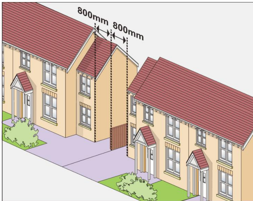
Diagram 12: Good side extension with 800mm retained between the sidewall of an extension and the plot boundary
