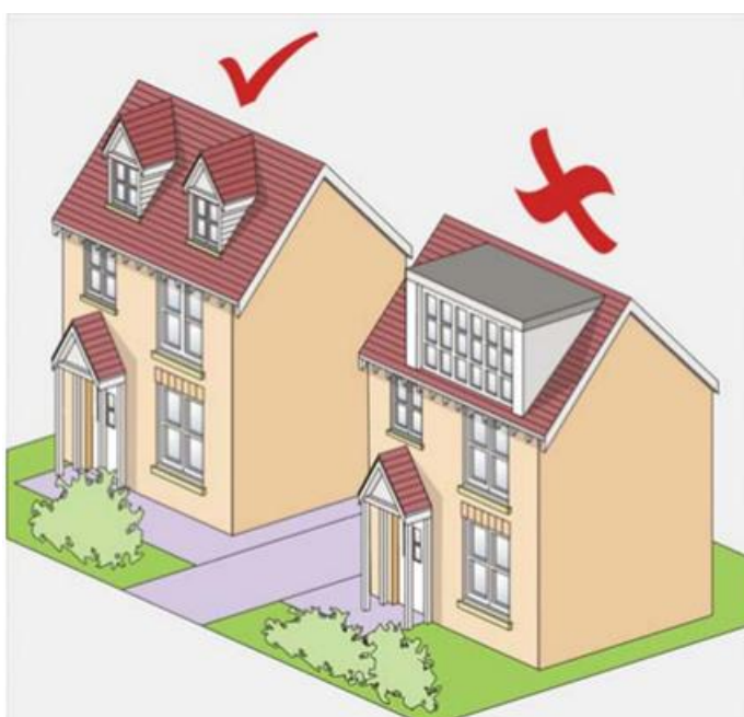
Diagram 18: Examples of dormer window extensions
